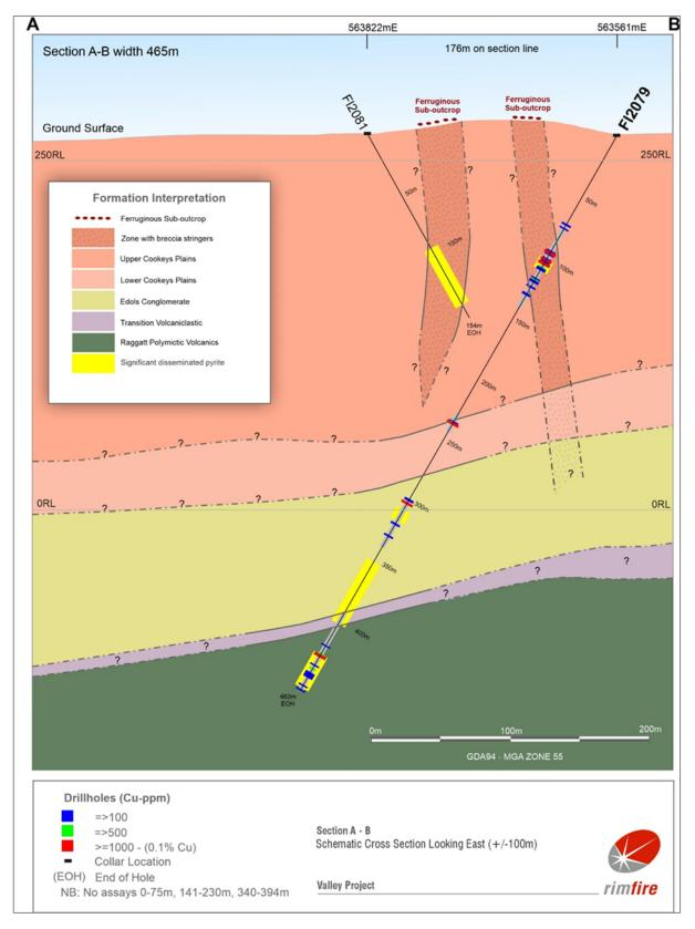
Figure 6: FI2079 and FI2081 Cross section showing Ordovician Raggatt Volcanics and copper anomalous breccia zones.
