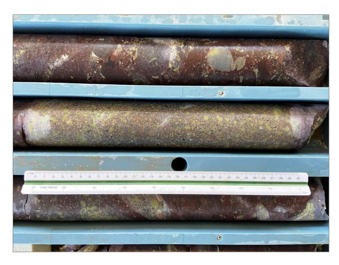
Figure 4: Epidote (green) and hematite (red) altered andesitic volcanic rock of the Raggatt Volcanics - FI2404 at 600 metres.
