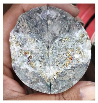
Figure 2: Disseminated bornite (copper iron sulphide) in calcite vein – Fl2405 at 376 metres.
