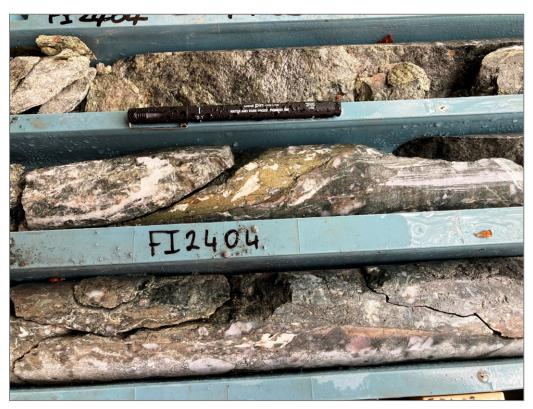
Figure 3: Stringer chalcopyrite (copper sulphide) in chloritic shear zone – FI2404 at 511 metres.
