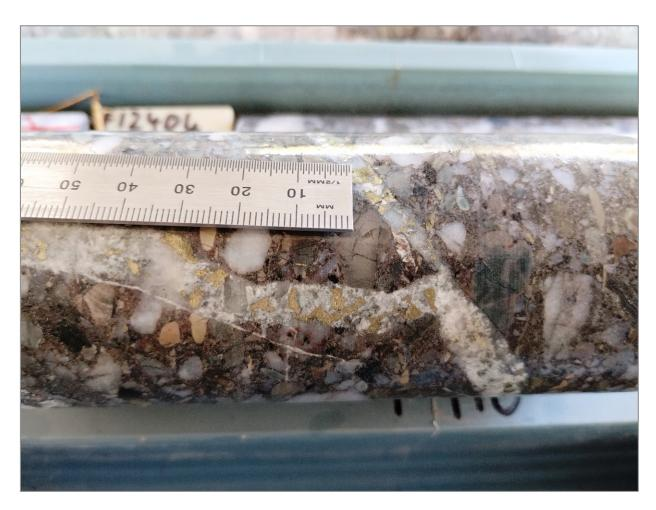
Figure 1: Coarse-grained blebby sulphide (chalcopyrite) in calcite vein – FI2404 at 469.4 metres.
