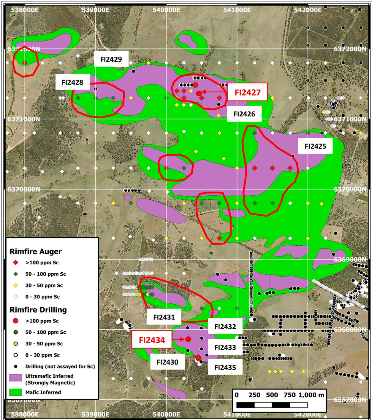
Figure 2: Murga drill collar plan (aerial photograph background image) showing, mafic / ultramafic intrusive units, Rimfire 2017 auger samples (coloured by scandium), Scandium in auger (+50ppm Sc) anomalies (red contours) and all Rimfire drill collars the majority of which have not been analysed for scandium.
