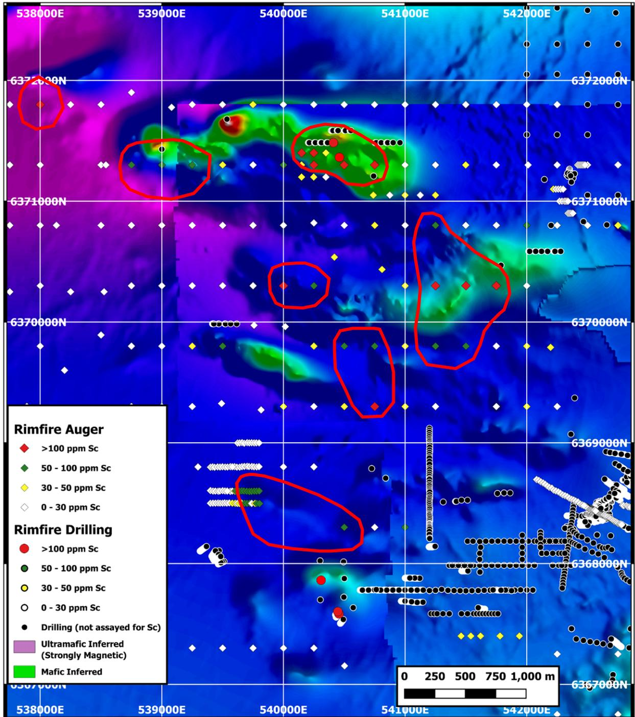
Figure 3: Murga drill collar plan (TMI background image) showing Rimfire 2017 auger samples (coloured by scandium), Scandium in auger (+50ppm Sc) anomalies (red contours) and all Rimfire drill collars the majority of which have not been analysed for scandium.
