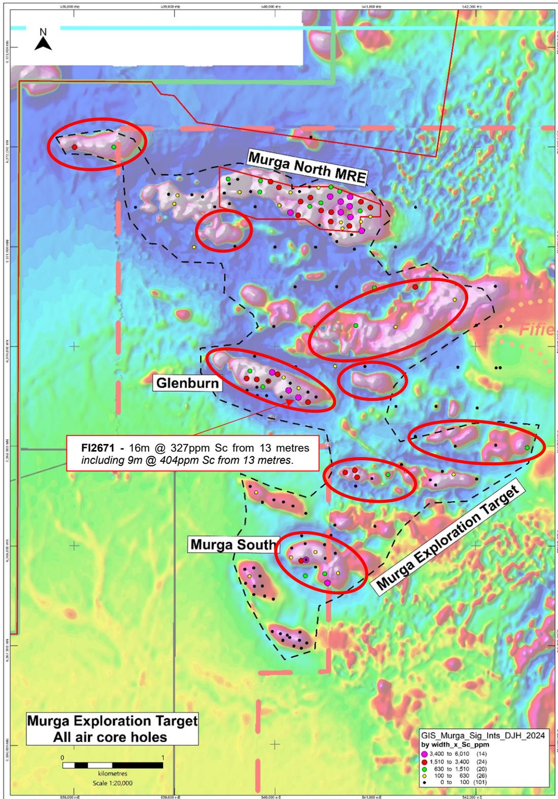
**Figure 3: Murga Exploration Target – all drill holes colour coded by scandium accumulation, i.e. intercept width multiplied by intercept grade. The method is useful in highlighting areas of greatest accumulation and areas for follow-up. Follow up areas highlighted by red polygons.**
