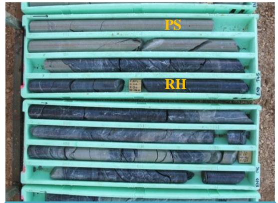
Porphyry Sill (PS) and Receptive Horizon (RH) in Fi 329 DDH
