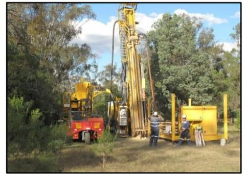
*RC Drilling at Roadside Area, Sorpresa*
