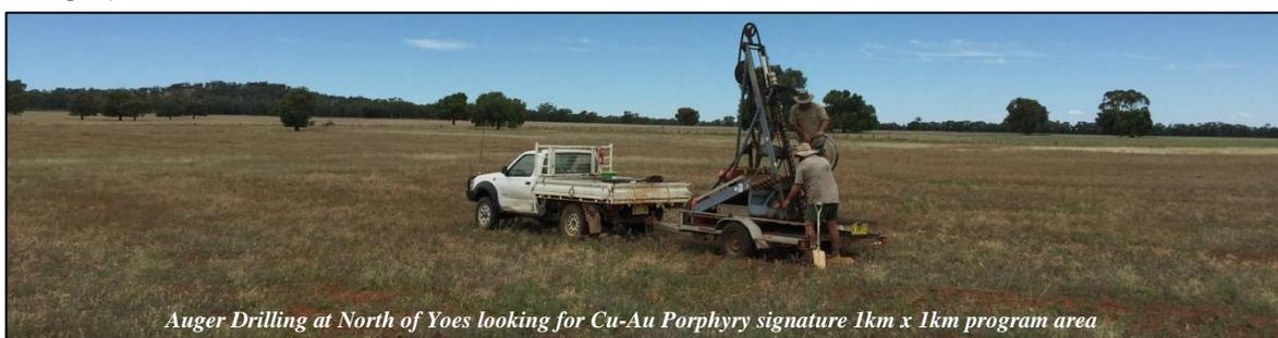
*Auger Drilling at North of Yoes looking for Cu-Au Porphyry signature 1km x 1km program area*
