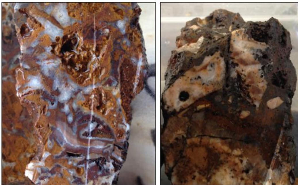
*Eclipse North Au – Ag – Base Metal (Cu-Pb-Zn) prospect, illustrating typical banded & brecciated, epithermal style, quartz vein float samples spatially associated with Au (>20ppb Au) in auger geochemical anomalies.*
