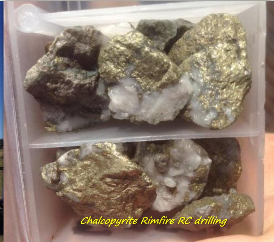
*Chalcopyrite Rimfire RC drilling*
