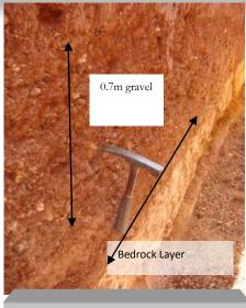
Gravel layer mined in Pit One Panel A & C
