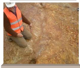
Examination the bedrock floor in Panel A, showing the fault lines now exposed, consistent with Trench 24 & 24A observations previously.
