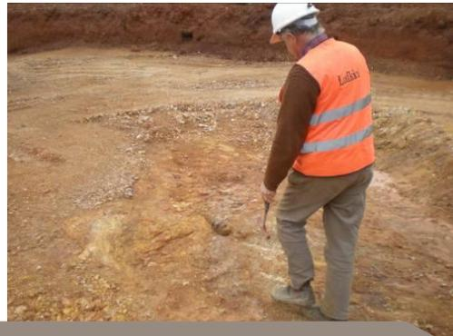
*Examination the bedrock floor in Panel A, showing the fault lines now exposed, consistent with Trench 24 & 24A observations previously. The bedrock system will be mined to a greater depth, then mapped and tested.*
