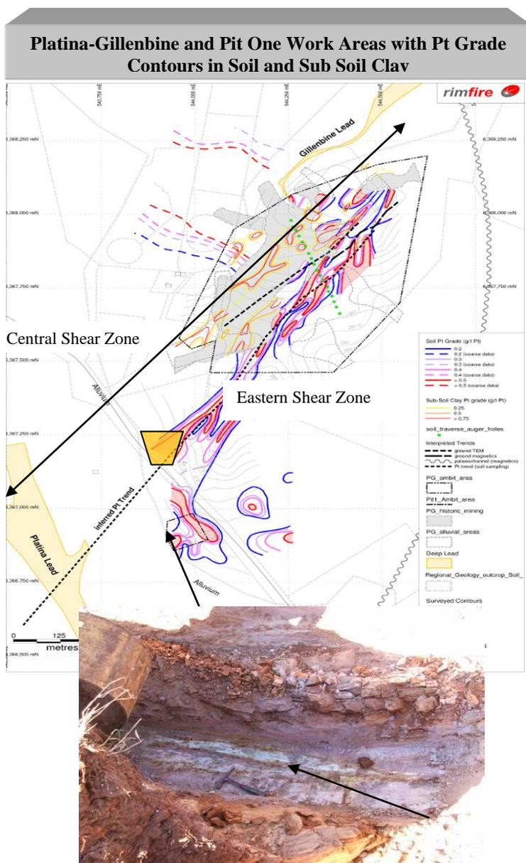
Base of Trench 24a Showing Pt bearing veins
