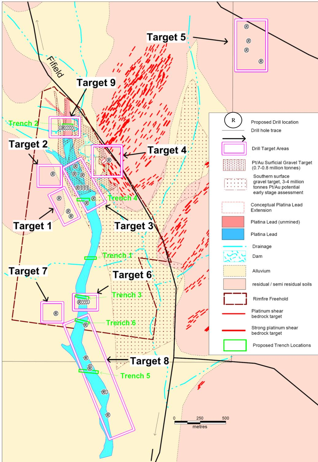
The map above denotes target areas that will be pursued with a combination of trenching and drilling in the Platina Valley location, principally centred on the Platina Lead structure.
