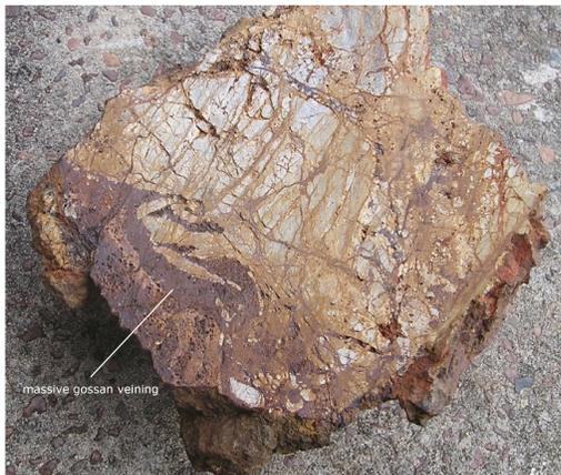
New Rock Chip Sample FiR203 sawn section of breccia showing massive gossan veining.
