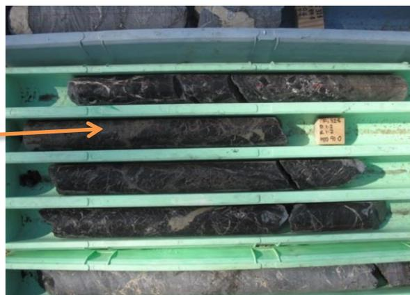
Fi 328 core shown from 90~93m depth – Spot XRF values on core surface include 1077 g/t Silver at 90.7m
