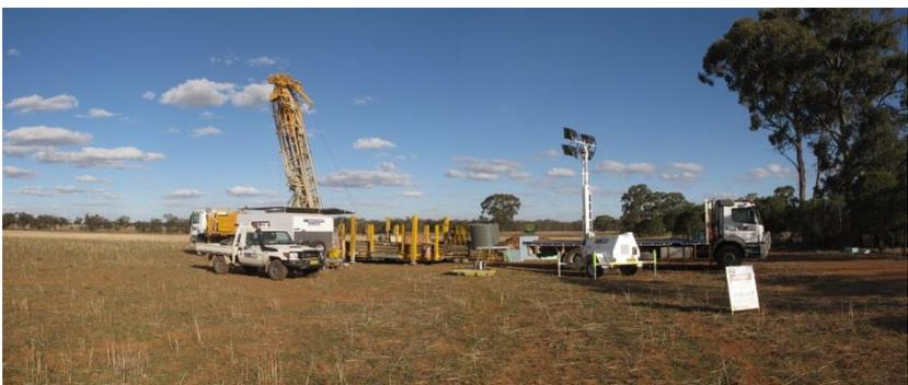
Diamond Drilling south east of Boundary Gate, core trays returning for examination
