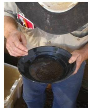
Loading the gravity plant with trial gravels and examining the precious metal concentrates to tune processing requirements
