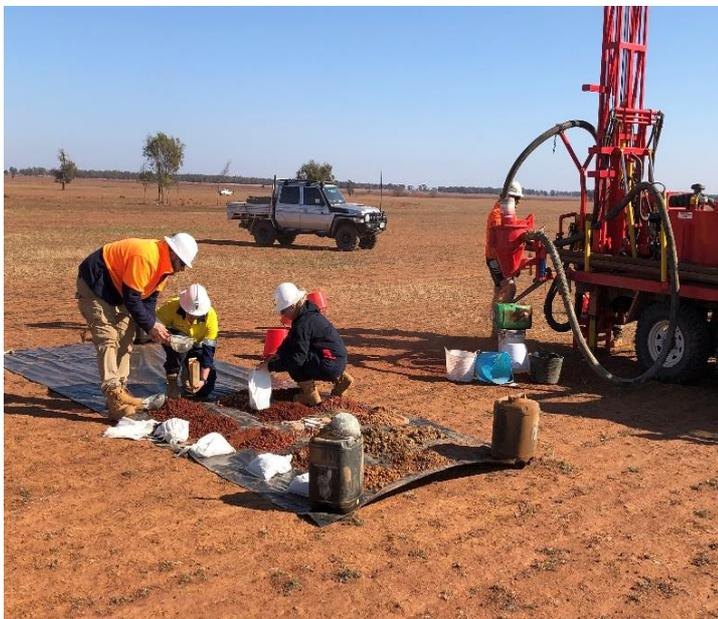
Aircore Drilling at Northern Area. Drilling technique requires no disturbance of topsoil and excess sample is placed back in hole on completion of sampling
