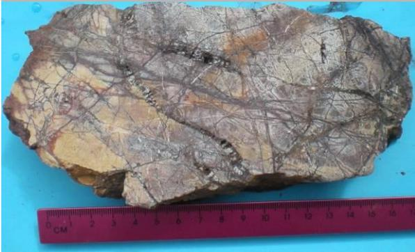
Gossanous brecciated in sediments
