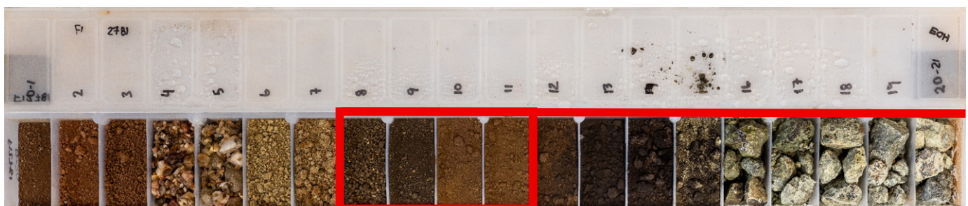
Figure 1: FI2781 chip tray photo with scandium intervals highlighted - 14m @ 194 ppm Sc (298ppm Sc Oxide) from 7m including 4m @ 338ppm Sc (518ppm Sc Oxide). Each compartment in chip tray represents a 1 – metre downhole interval.
