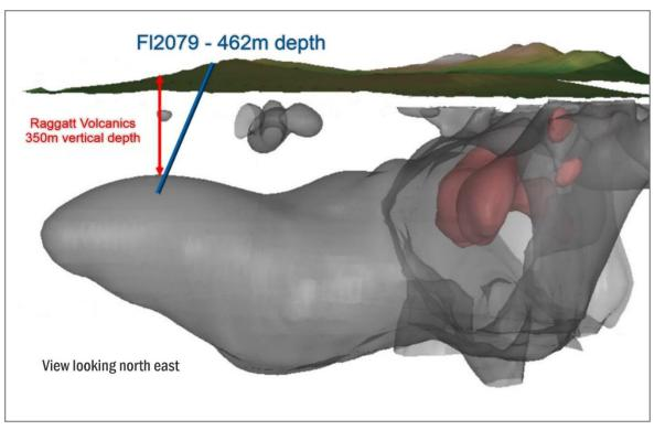
Interpreted magnetic model of Ordovician rocks (in grey), which was tested by drilling and verified with Ordovician rocks occurring under younger sediment package at around 350m vertical depth.
