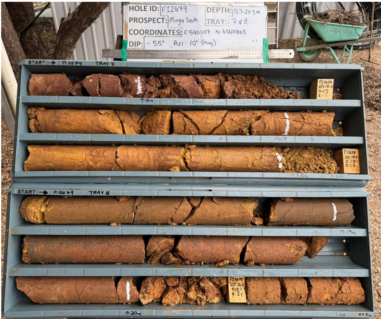
Figure 5: Photo of FI2679 PQ core – 15.7 to 20.5 metres (clay rich laterite)
