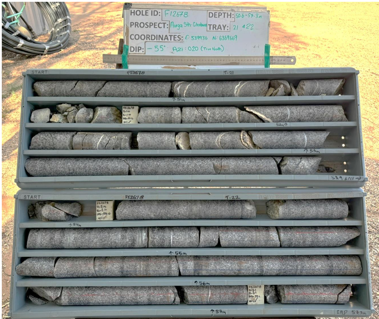
Figure 4: Photo of F12678 HQ core – 50.6 to 57.3 metres (coarse grained pyroxenite)
