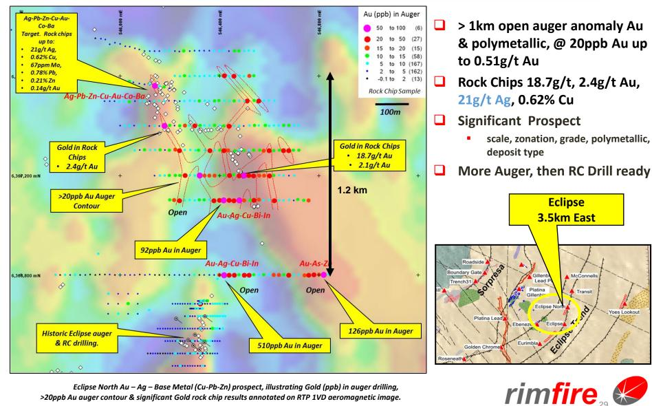
Eclipse North Au – Ag – Base Metal (Cu-Pb-Zn) prospect, illustrating Gold (ppb) in auger drilling, >20ppb Au auger contour & significant Gold rock chip results annotated on RTP 1VD aeromagnetic image.
