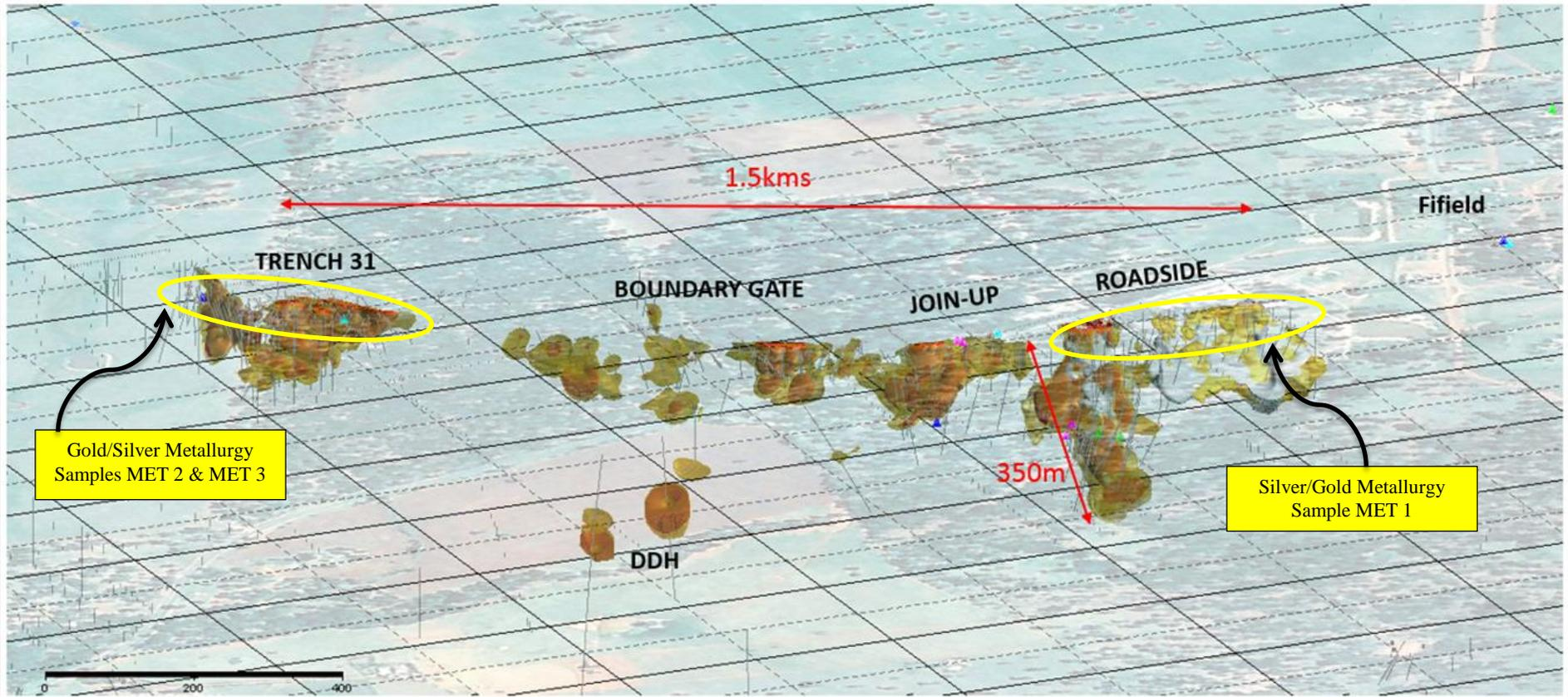
The metallurgy sample locations are shown on the Sorpresa main project area. Samples were taken in the 0~45m oxide zone, in three locations at Trench 31 (MET 2) & Trench 31 South West (MET 3) and also the Roadside (MET 1) location.
