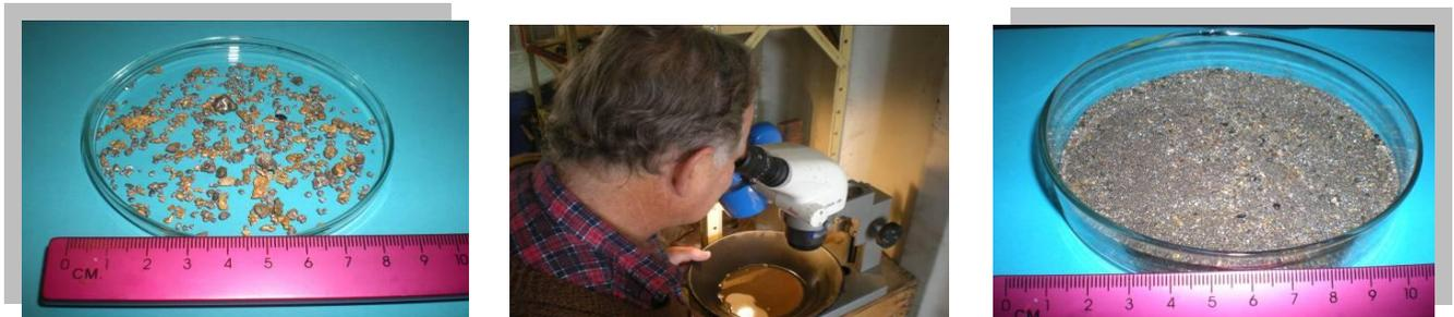
*Examining clean precious metal concentrates where coarse (left) and fine (right) Pt and Au have been recovered, with selected material being refined (approx. 400g) or undergoing further petrological testing.*
