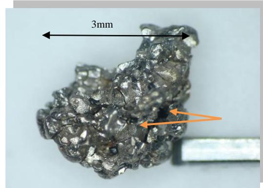
*Short travelled Pt Grain, angular and indented with unidentified intergrown mineral inclusions*
