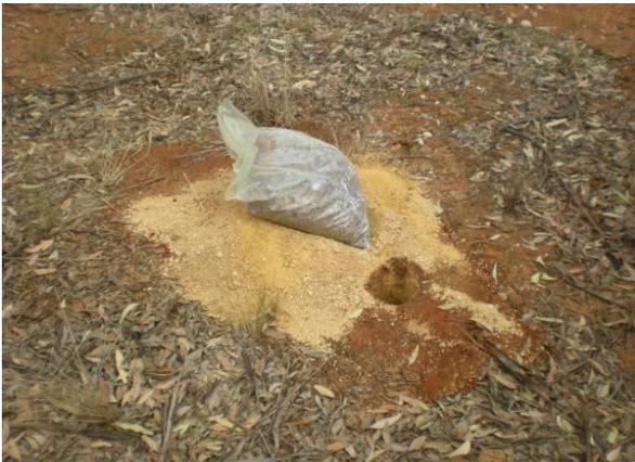
*Auger drilling to determine gravel locations, thickness and the bedrock valley floor with possible tributaries to the historic Platina Deep Lead.*
