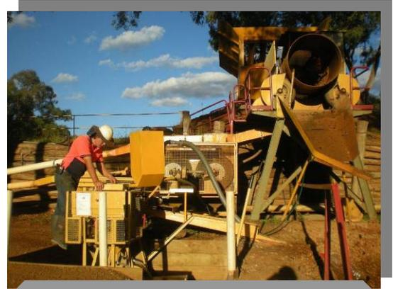
*Gravity Plant able to process in excess of 100mt/day of low clay gravels, when operational*
