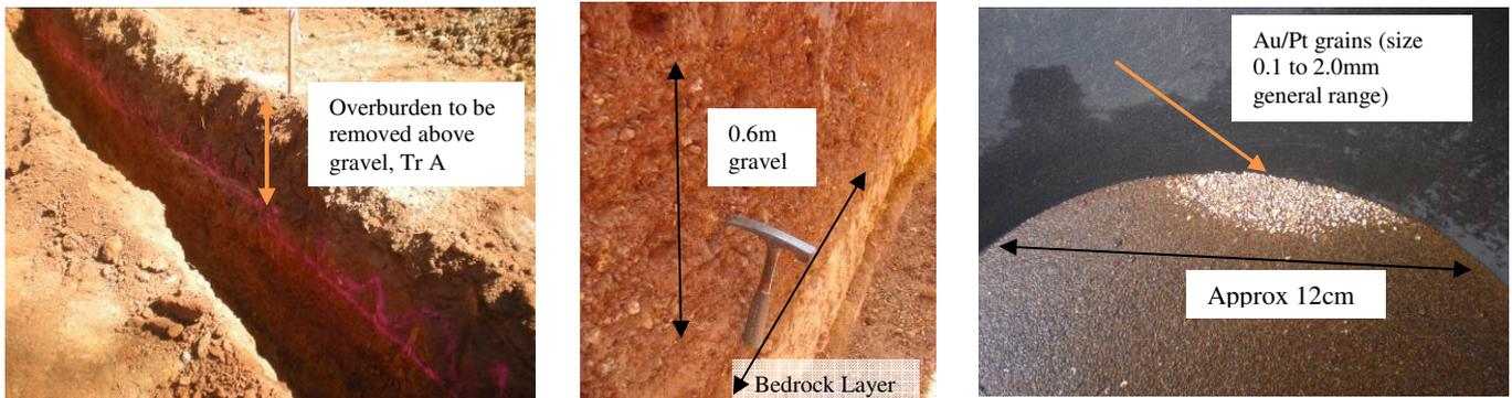
*Tr A within Pit One intersected gravel, which has been processed and is yielding Au/Pt grains (no quantitative grade yet established)*
