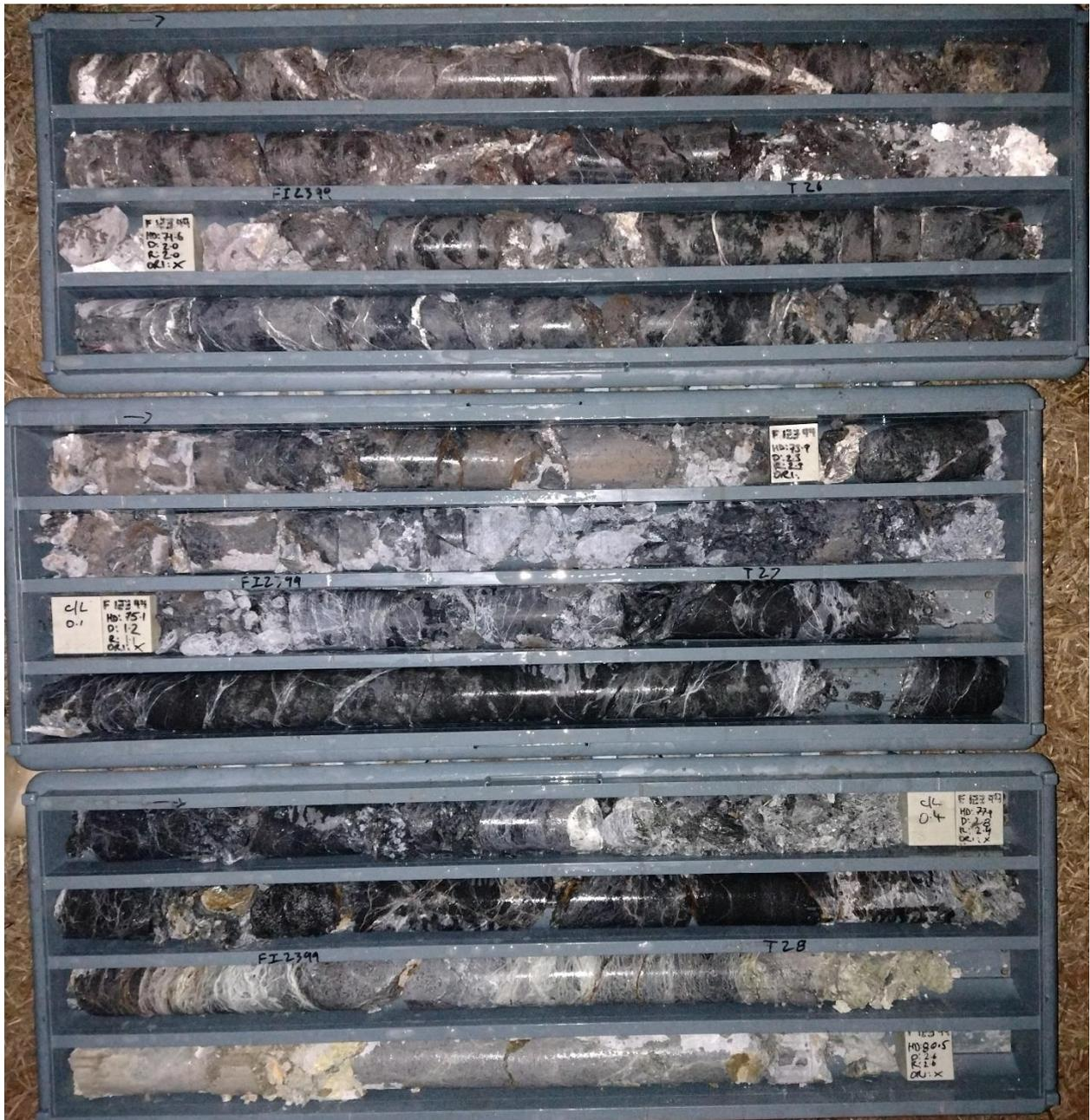
Figure 5: Photo of drill core from Melrose drill hole FI2399 - 70 to 80.5 metres downhole). Ultramafic rock types – dunite (black) and pyroxenite (grey).
