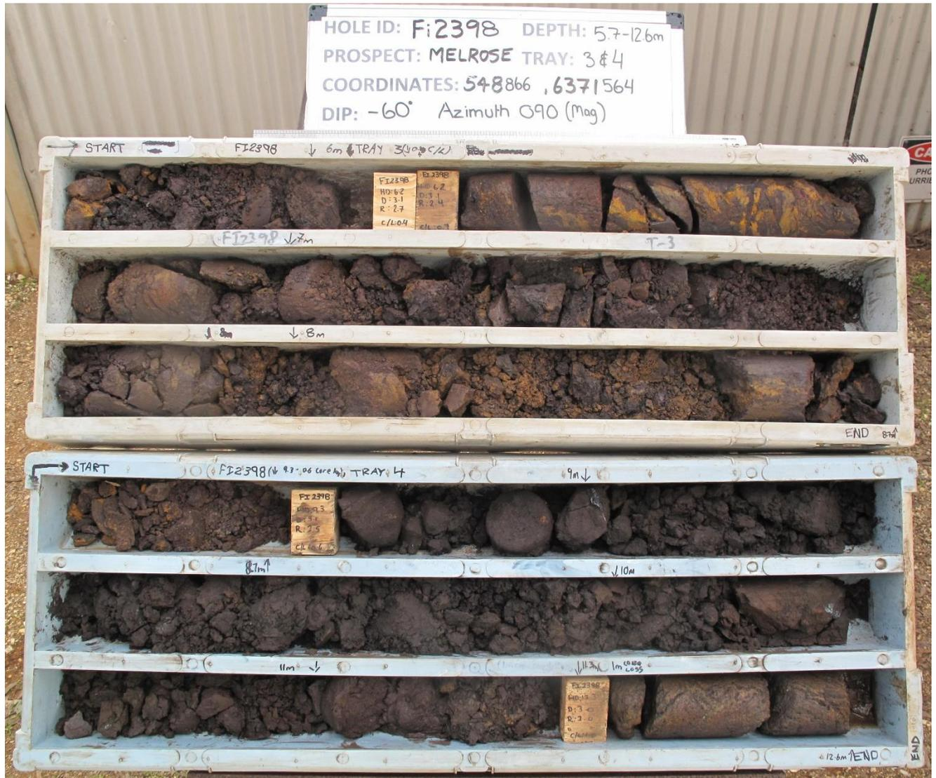
Figure 4: Photo of drill core from Melrose oxide nickel – cobalt – scandium – platinum zone (FI2398 5.7 to 12.6 metres downhole).
