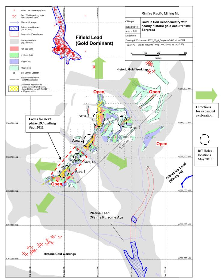
Appendix 2 RC Drilling at Sorpresa Gold Project – 15 Holes designed to Extend Area 1
