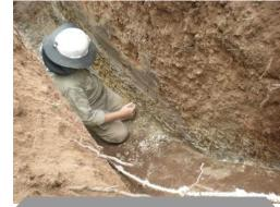
Bedrock breccia zone now exposed in a 10m trench located on an Auger traverse section FiAug 822~824 with encouraging Au assay
