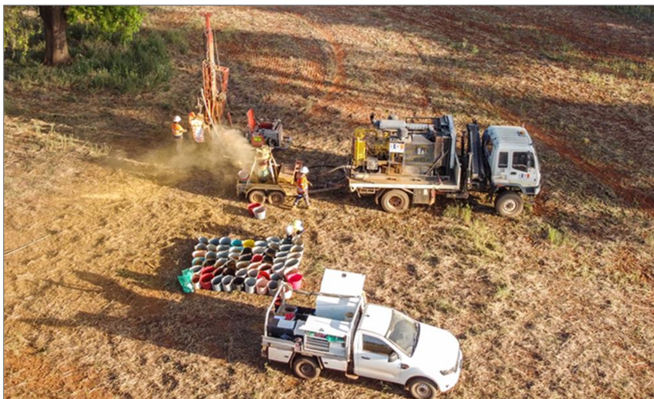
Figure 1: Rimfire aircore drilling underway at the Currajong cobalt prospect
