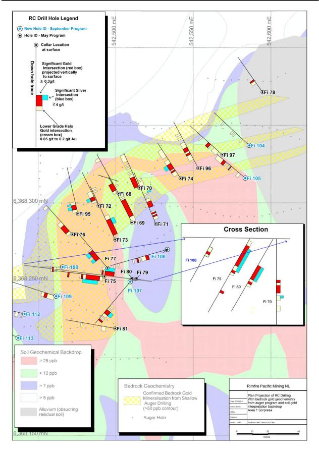
Area 1 (North) - September 2011 RC Drilling showing Au and Ag intersections in Plan View
