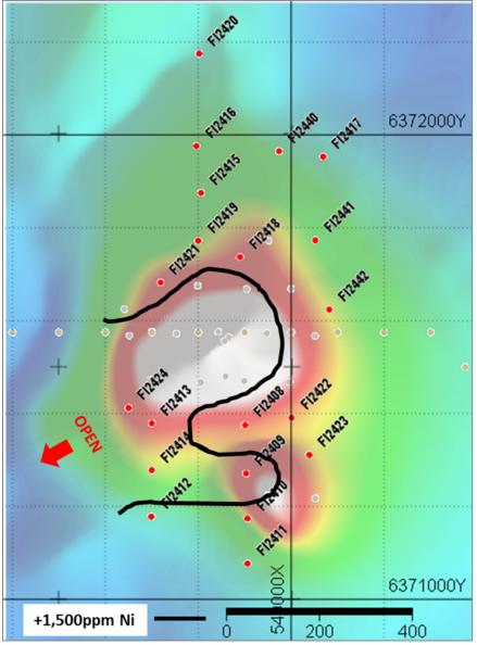
Figure 4: Melrose prospect – nickel in laterite zone (as shown by +1,500ppm Ni contour) which remains open to the southwest.
