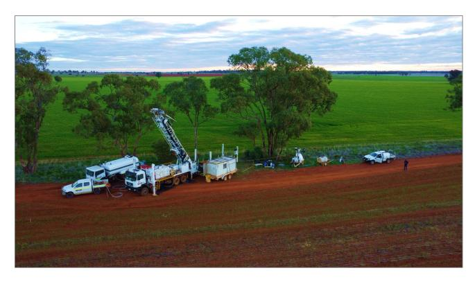
Figure 1: Diamond drilling operations underway at the Melrose prospect. Note the drill rig has been positioned along a fence to avoid damage to fresh crops.
