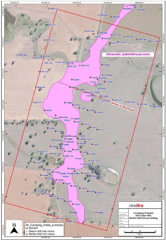
Figure 4: Currajong prospect drill collar plan showing Rimfire 2022 air core drill hole collars (red) and hole ID's.
