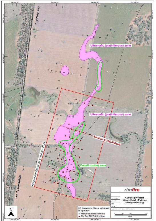
Figure 3: Currajong prospect drill collar plan showing Rimfire 2022 air core drill hole collars (red) and historic drill hole collars (black circles), platiniferous ultramafic and cobalt (200ppm Co) zone.
