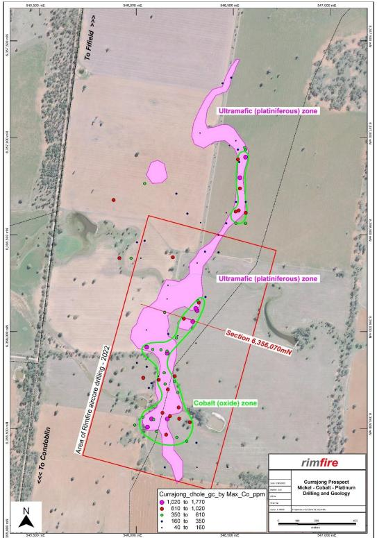
Figure 5: Currajong prospect drill collar plan showing Rimfire 2022 aircore drill hole collars color – coded by maximum downhole cobalt (ppm), and cobalt (200ppm Co) zone.
