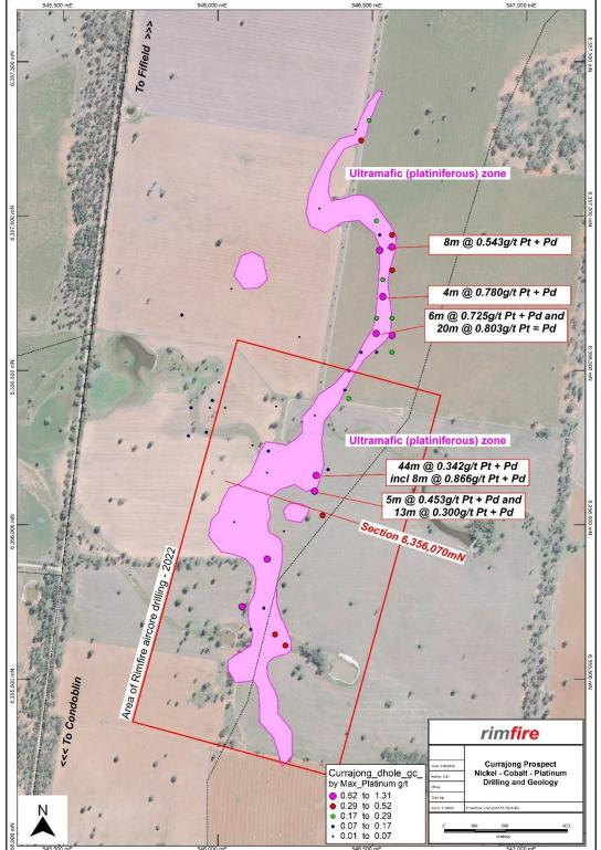
Figure 6: Currajong prospect drill collar plan showing Rimfire 2022 aircore drill hole collars color – coded by maximum downhole platinum (ppm), and cobalt (200ppm Co) zone.
