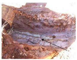
Base of Trench 24a Showing Pt bearing veins
