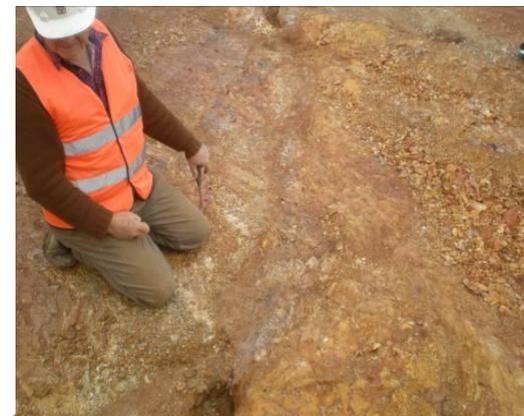
*Examination the bedrock floor in Panel A, showing the fault lines now exposed, consistent with Trench 24 & 24.A observations previously.*
