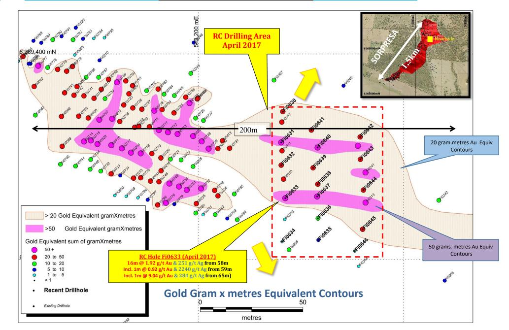
Figure 5: RC Drilling at Sorpresa – Roadside Area - showing gram-metre in plan view Au Eqivalent (1gm Au = 70gm Ag conversion)
