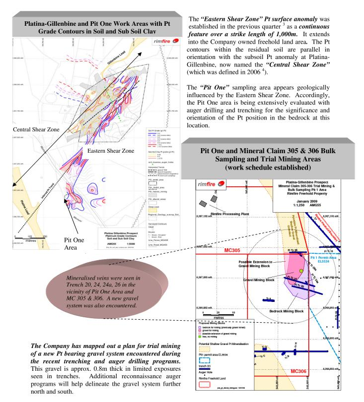
The overburden will first be removed  $(1\sim 2m)$ , the gravel will be trial mined and the bedrock will be cleaned off over the entire area, mapped and sampled. The bedrock will be tested with layered exposures created in "plan
