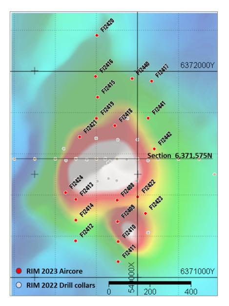
Figure 2: Melrose drill collar plan (TMI image) showing Rimfire's 2023 aircore drill collars (red) and previous Rimfire drill collars.
