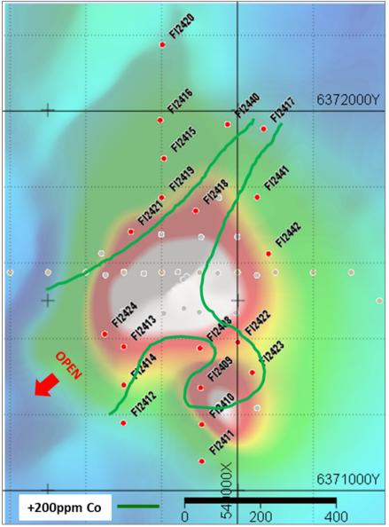
Figure 5: Melrose prospect – cobalt in laterite zone (as shown by +200ppm Co contour) which remains open to the southwest.
