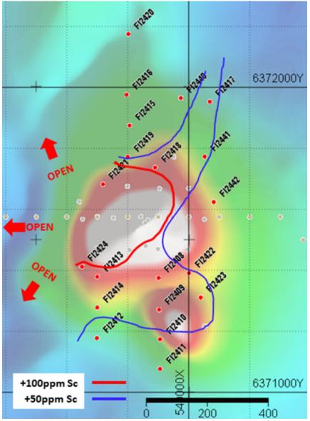
Figure 6: Melrose prospect – scandium in laterite zone (as defined by +50ppm and +100ppm Sc contours) which remains open to the west.
