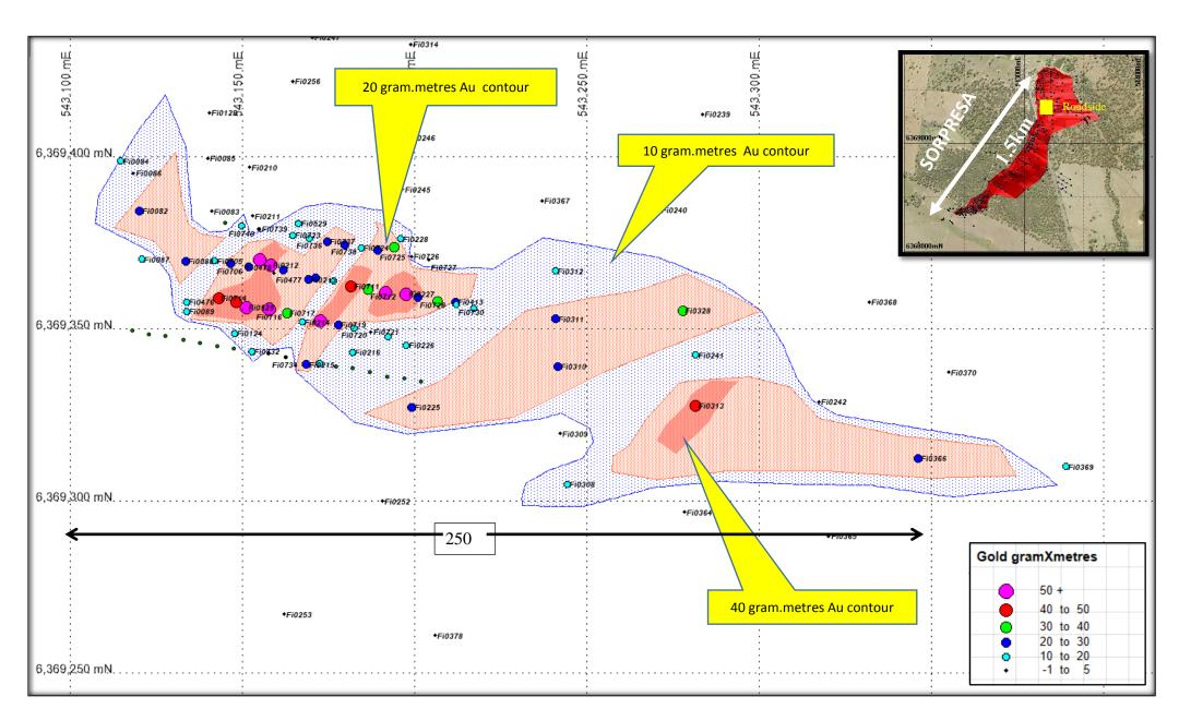
Figure 4: RC drilling at Sorpresa - Trench 31 Area Oxide - Gold in Gram-Metre Representation with some recent highlights >50 gram-metre shown
