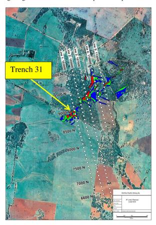
The survey consisting of 5 lines (total approx.12km) at Sorpresa, with 100m electrode spacing separations and will be completed and analysed within the first quarter 2012.
