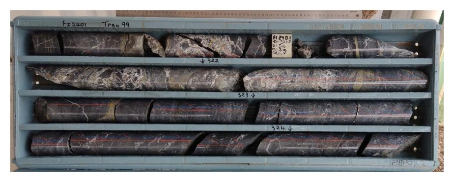
Close up of diamond drill core with gold mineralised carbonaceous shale ("Sorpresa Beds") (FI2401 - 321 to 324 metres)
