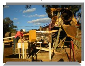
Gravity Plant able to process in excess of 100mt/day of low clay gravels, when operational
