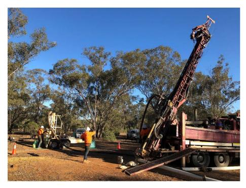
The Aircore drilling at the Northern and Southern Area prospects is designed to obtain bedrock regional lithological, geochemical and alteration samples from the highly prospective Northern (40km<sup>2</sup>) and Southern (100km<sup>2</sup>) areas where there is potential for a significant size (> 1Moz gold +/- 1Mt copper) discovery.
