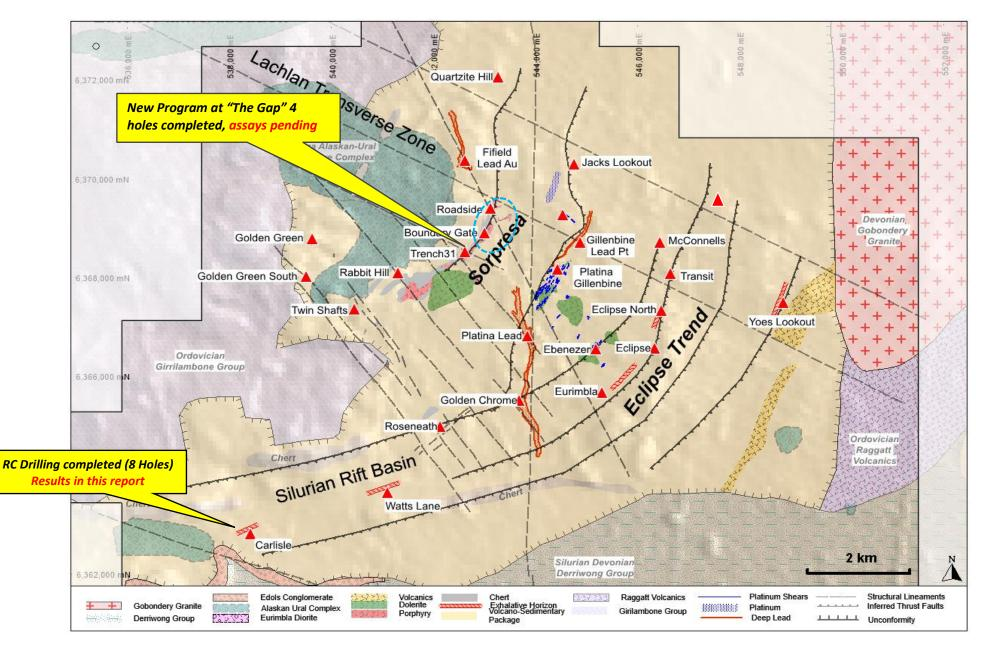
*Example 2: Carlisle Target 1 – RC drill hole location plan illustrating high grade rock chips, drill intersections on Aeromagnetic Image (RTP 1VD). A tight structural and lithological control to mineralisation is evident striking to the NE.*
