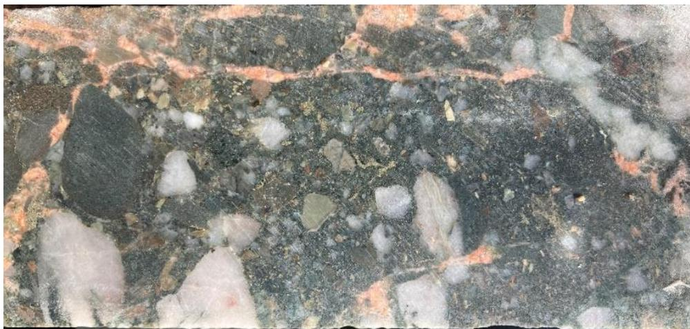
**Figure 7:** FI2079 core photo at 440.35m: Spectacular Ordovician volcanioclastic polymictic conglomerate with strong propylitic epidote altered groundmass and selectively pink hematite dusted pebbles. This style of alteration is typical of the mineralised Ordovician. Minor disseminated and vein-controlled pyrite is associated with the epidote alteration. Epidote can comprise up to 20% of the rock volume.
