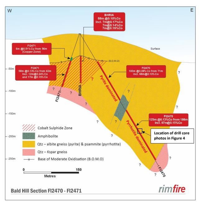
Figure 3: Bald Hill cross section looking to NNE. Note that the geological relationship between FI2470 and FI2471 and BHR1A is unknown at this stage. Refer to Figure 2 for section locations.
