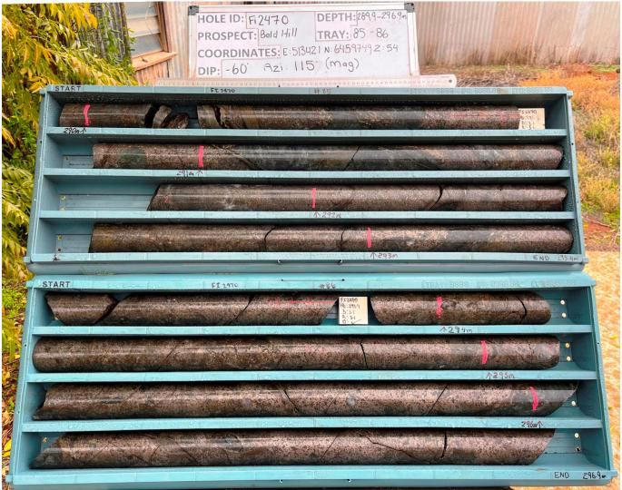
Figure 4: Sulphide rich diamond drill core from FI2470 289.9 – 296.9 metres. Red lines on the drill core show the start and finish of each 1-metre interval. Down hole depth is shown on the core tray edges, and Individual (1 metre) assay cobalt grades are shown below in Table 2.
