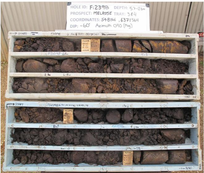
Figure 4: Photo of drill core from Melrose oxide nickel – cobalt – scandium – platinum zone (FI2398 5.7 to 12.6 metres downhole).
