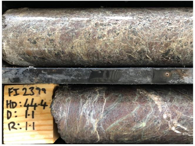
Figure 6: Photo of drill core from Melrose drill hole FI2399 – 44.4 metres downhole. Strong hematite alteration in ultramafic rock.
